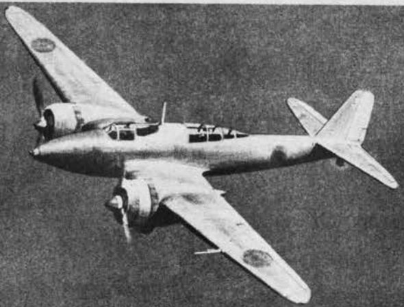
Randy , new Jap fighter, resembles Nick but has cleaner greenhouse, flat-topped tail, longer nacelles protruding past the wing's trailing edge.
